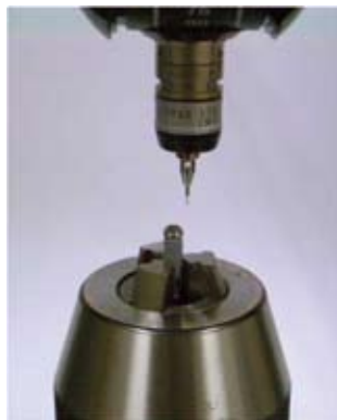
Figure 1: Implant component feature measurement by ruby probe tip of CMM
